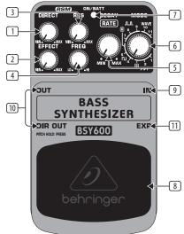
frequency moves (DECAY). When the decay time is set to MAX, the cut-off filter frequency is fixed.
